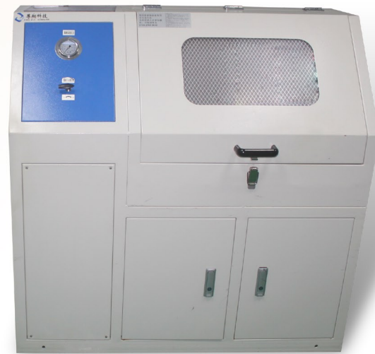
WATER HAMMER BLASTING
